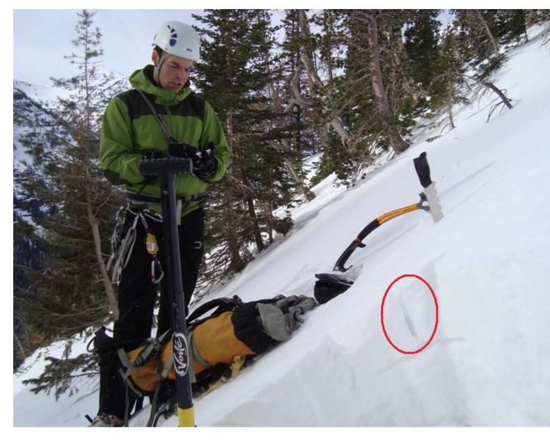
Mark Staples investigates cracks in the snow near the edges of the gully. The circle shows the crack from the avalanche. The slope above the fracture settled and cracked as we approached. A thick layer of unconsolidated facets was loaded with a dense, 1 finger to pencil hardness wind slab.
