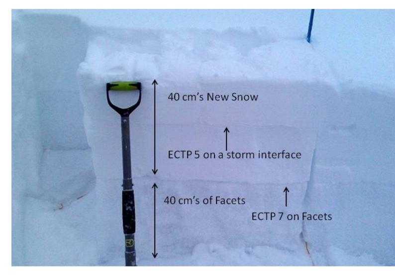
Over the past three days a heay load was deposited on a very weak foundation. Stability tests produced unstable results both within the storm snow and on the new snow/old snow interface. Dangerous avalanche conditions exist on Mt Ellis. Photo GNFAC
