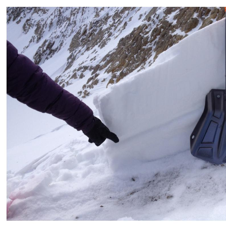
This broke on facets formed during two weeks of cold weather. It broke 6-12 inches deep, about 100 feet wide and ran about 300 feet vertical. Photo: GNFAC
